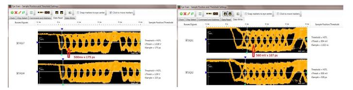
DDR4 Read and Write Bursts as seen by the Keysight U4154 at the FS2510 interposer
