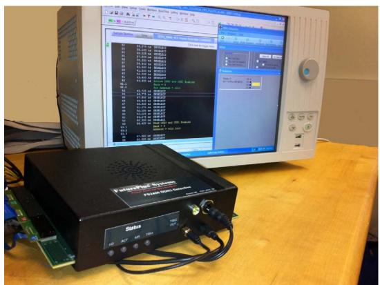
**Figure 8** : When used in conjunction with a logic analyzer the *DDR3 Detective*<sup>TM</sup> can show the DDR Data bus traffic around the error in addition to the Address/Command/Control signals.
