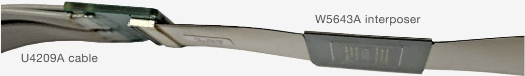
Bottom side view of the cable/interposer attachment
